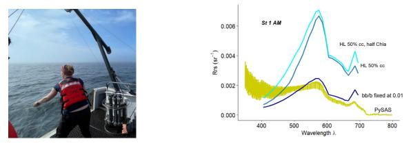
**Picture** *left*: Deployment of the profiling radiometer Hyper-Pro during the scientific half-day cruise in Harpswell Sound and the Gulf of Maine (photo by: Meredith Kime). *right*: Observed PySAS remote sensing reflectance ( $R_{rs}$ ) in comparison to three modelled spectra from Hydrolight simulations based on IOP data acquired on the cruise. We hypothesised after our analysis, that the backscattering ( $b_b$ ) had been overestimated by the in-situ IOP instrument (BB9).
